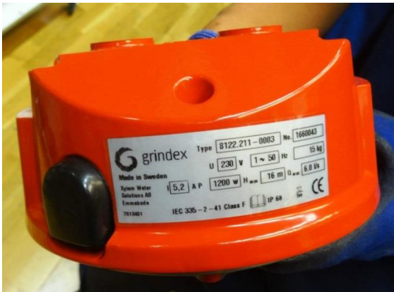
Data plate outside the pumptop
