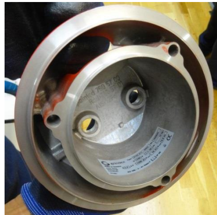
Data plate inside the pumptop
