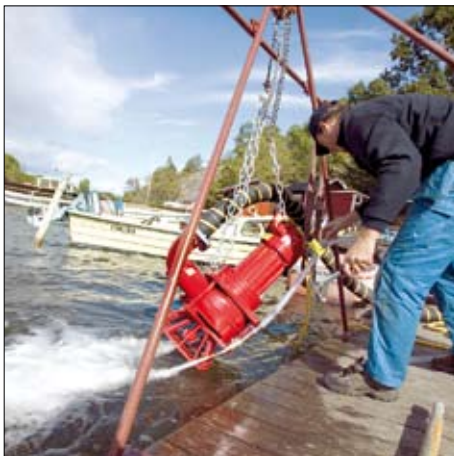
When dredging, the slurry pump can be equipped with external water jets to stir up settled solids.
